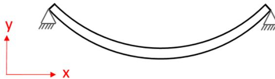
Figure 4.2.3. Boundary Conditions for Laminate Composite Leaf Spring Model
