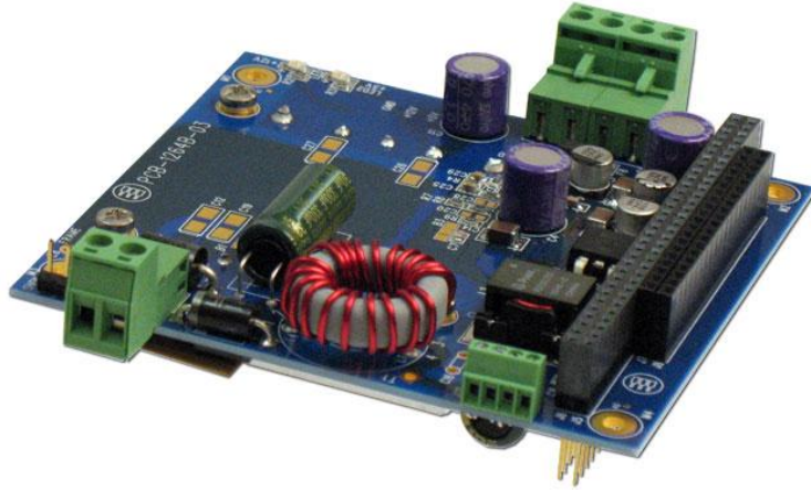
Figure 1.3. Discrete Type Isolated DC/DC Converter (after [5])
