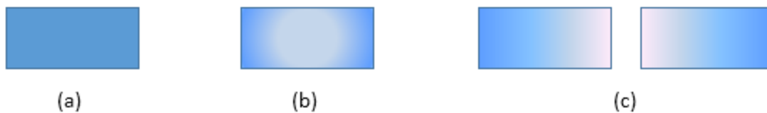
Figure 2.8. Visual Representation of the Effect on Current Density Distribution in the Cross-Section of the Transformer Coil: (a) DC, (b) Skin Effect, and (c) Proximity Effect
