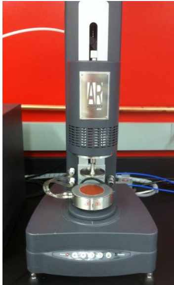
Figure 3-4: TA Instruments AR2000EX used in this study, shown in parallel plate configuration.
