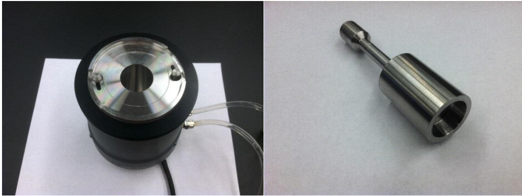
Figure 3-5: Cup-and-bob geometries used in study
