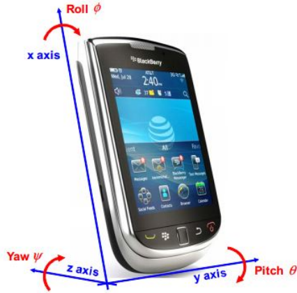
Figure 3.2: Device Coordinate System & Axis of Rotations
