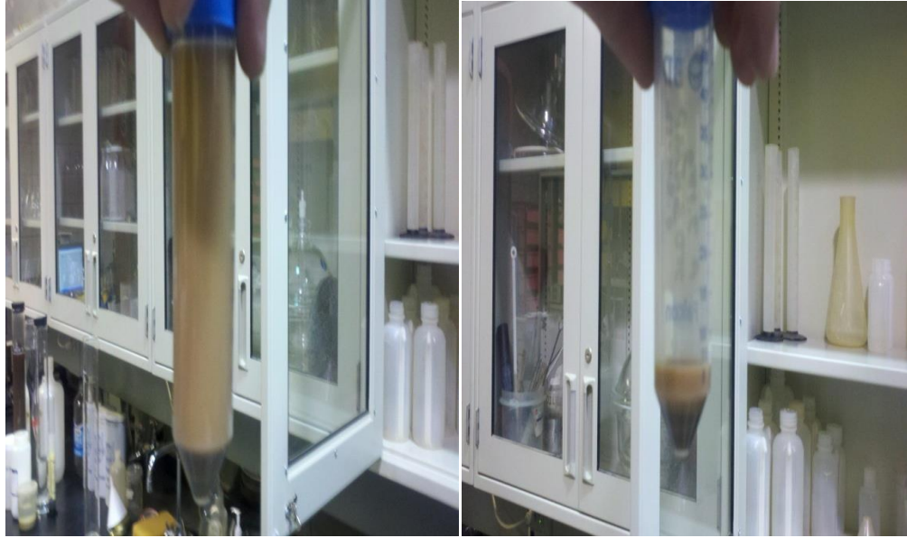
Figure 40: Separation of clay fraction from silt fraction
