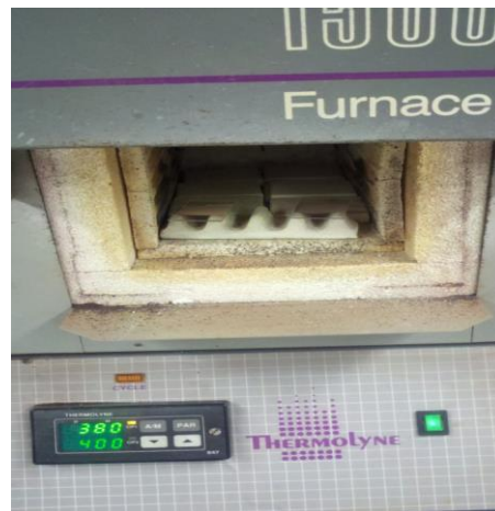
Figure 38: Muffle furnace used for heat treatments
