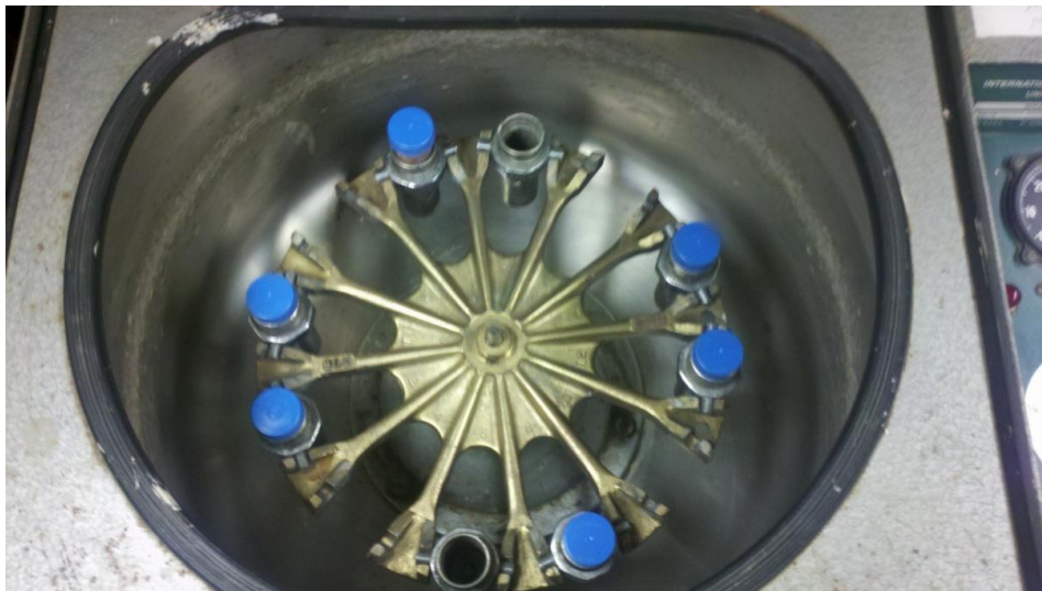
Figure 39: Centrifuge used for particle separation
