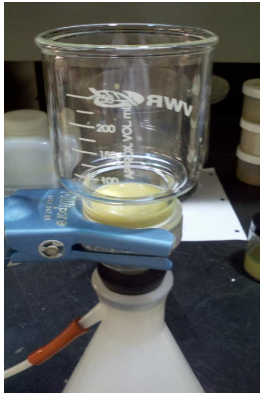
Figure 33: Sample being filtered on a Millipore filter
