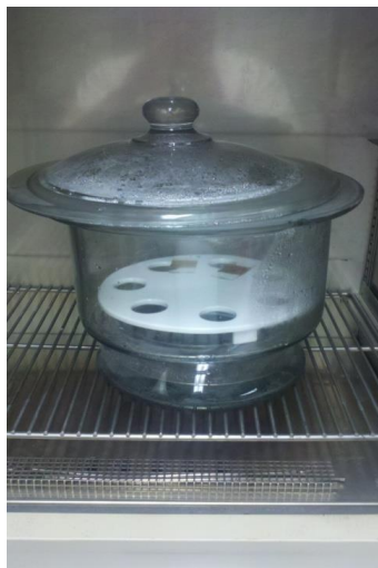
Figure 37: Sample in adsorption treatment of Ethylene Glycol
