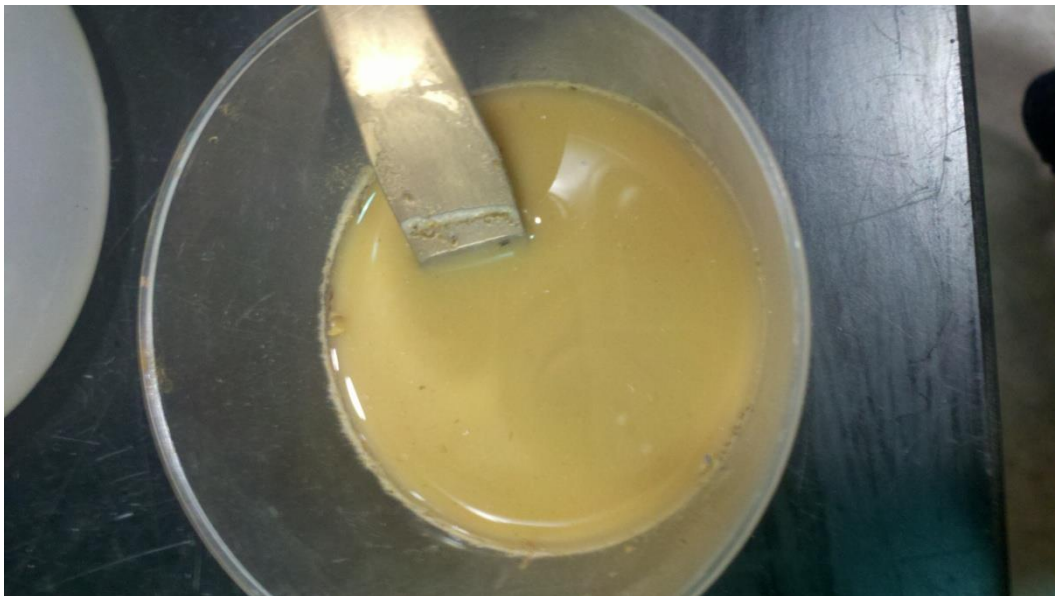
Figure 32: Slurry of soil and sodium hexametaphosphate solution
