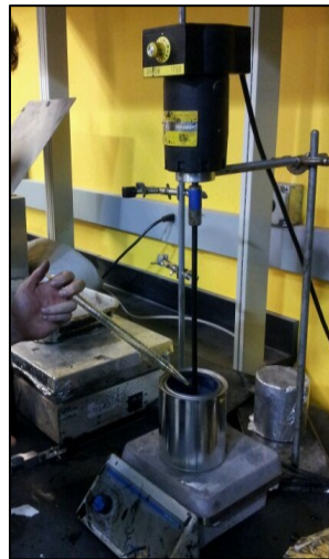
Figure 3-3 Adding Evotherm™ to Control Asphalt Binder
