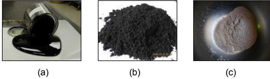
Figure 2-1 (a) Soft Asphalt Binder (b) Fine Crumb Rubber (c) AMBS (Source: Consulpav 2013)
