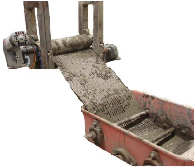
Figure 1.6 Pultrusion setup with motors attached to the rollers
