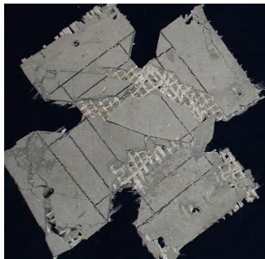
Figure 3.44 Crack pattern for Textile 2 – S1 – T2 - 0°
