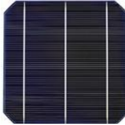
Figure 35: Silver Grid Contact Design for SPL Cells
