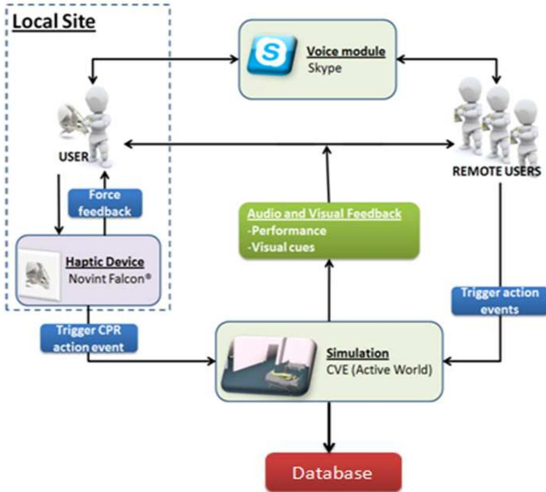
Figure 4.5: System design - ACLS training simulator using ActiveWorlds.
