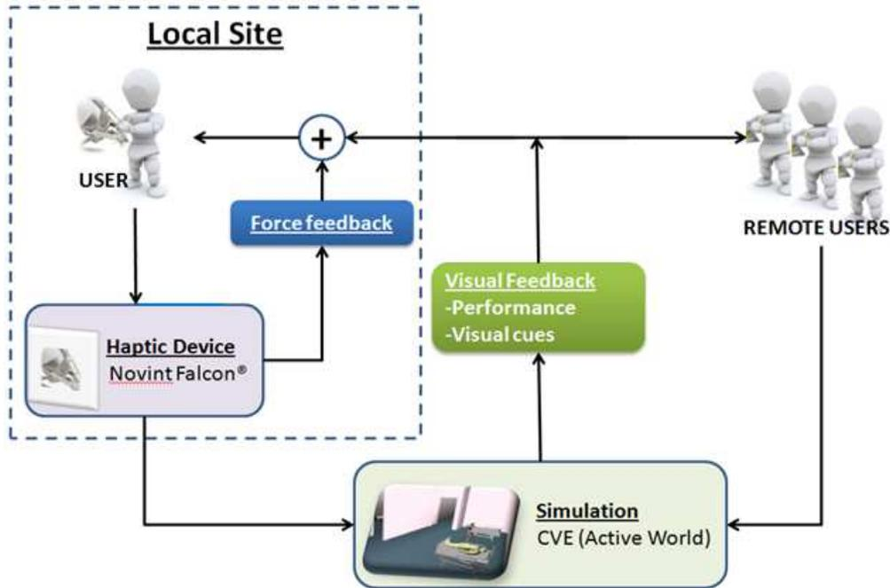
Figure 4.1: System Design - CPR training simulator in ActiveWorlds®
