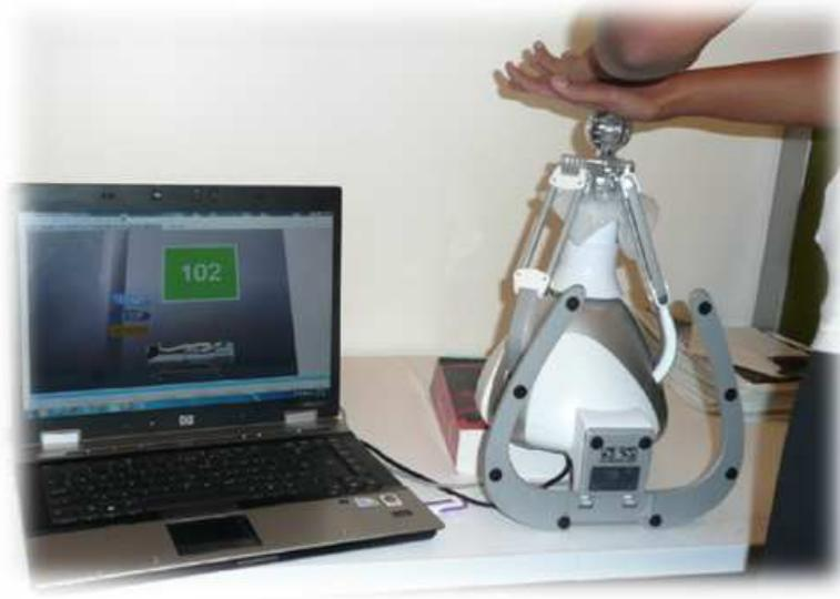
Figure 4.3: Experiment Setup: CVE shown at the left and haptic device at the right.
