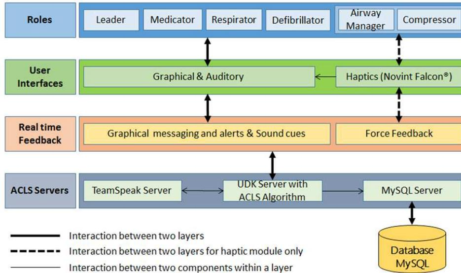
Figure 5.2: System architecture of the VR-based ACLS training simulator.
