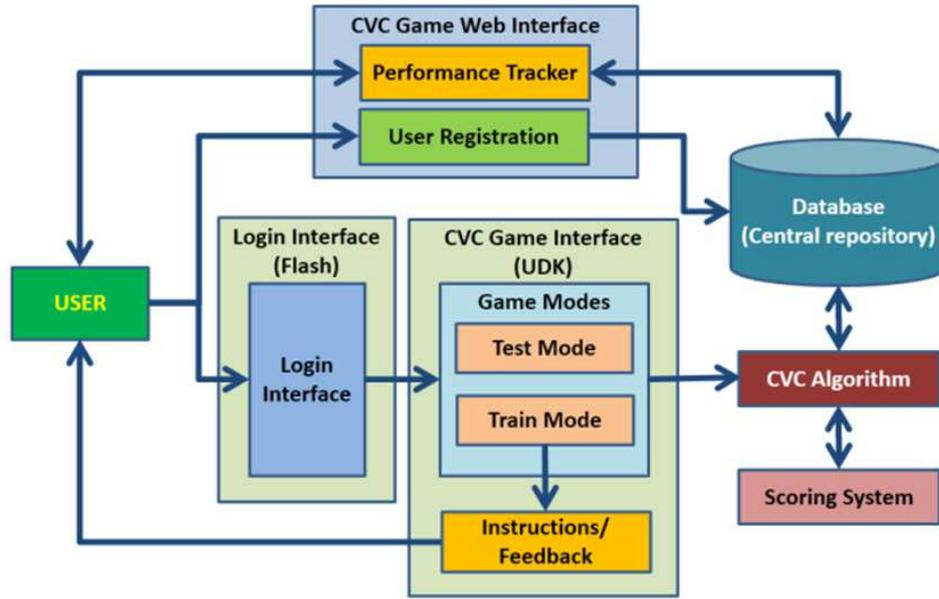
Figure 4.10: System design of the Central Venous Catheter placement simulator.
