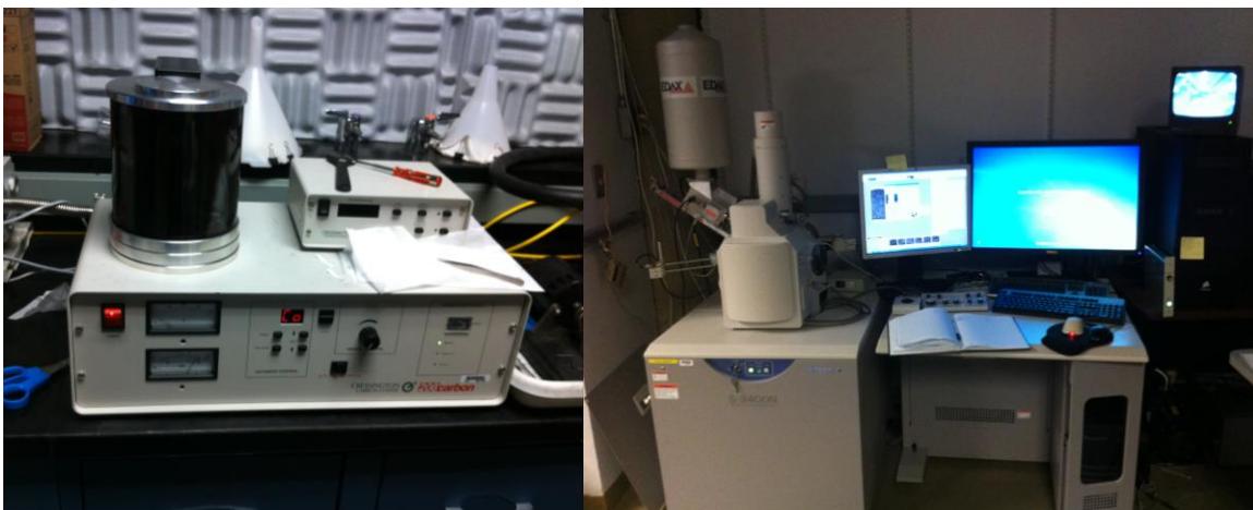
Figure 3.2.1.3. (a) Carbon coater; (b) The HITACHI S-3400 electron scanning microscope used for the microstructural study
