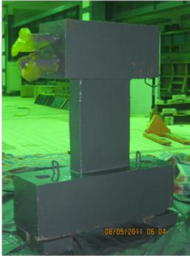
Figure 7.3.1.3. The CHMC retrofitted RC shear wall specimen
