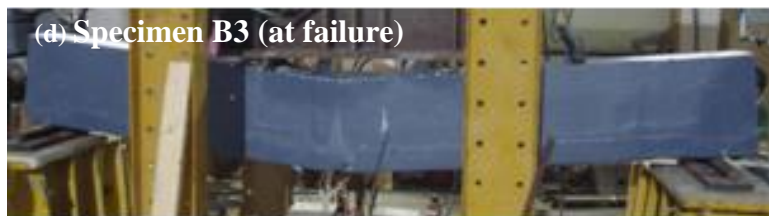
Figure 6.2.4.1. Experimental test results and failure modes of the SRC girders
