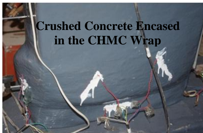
Figure 7.3.2.4. close-up view of the confined region near the base of the wall right before the test was stopped
