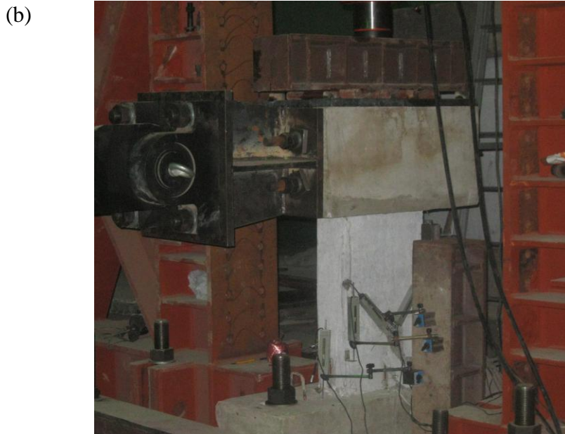
Figure 7.2.1.2. Experimental setup and instrumentation: (a) schematic figure; (b) picture
