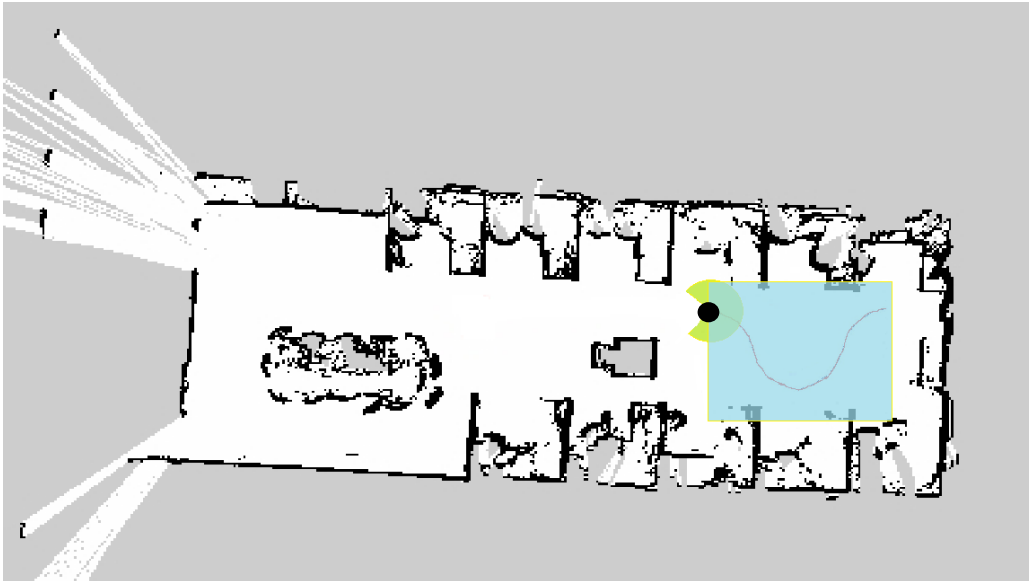
Figure 12. Path through an area that's supposed to maximize area covered. Robot position and the field of view circle are approximate.
