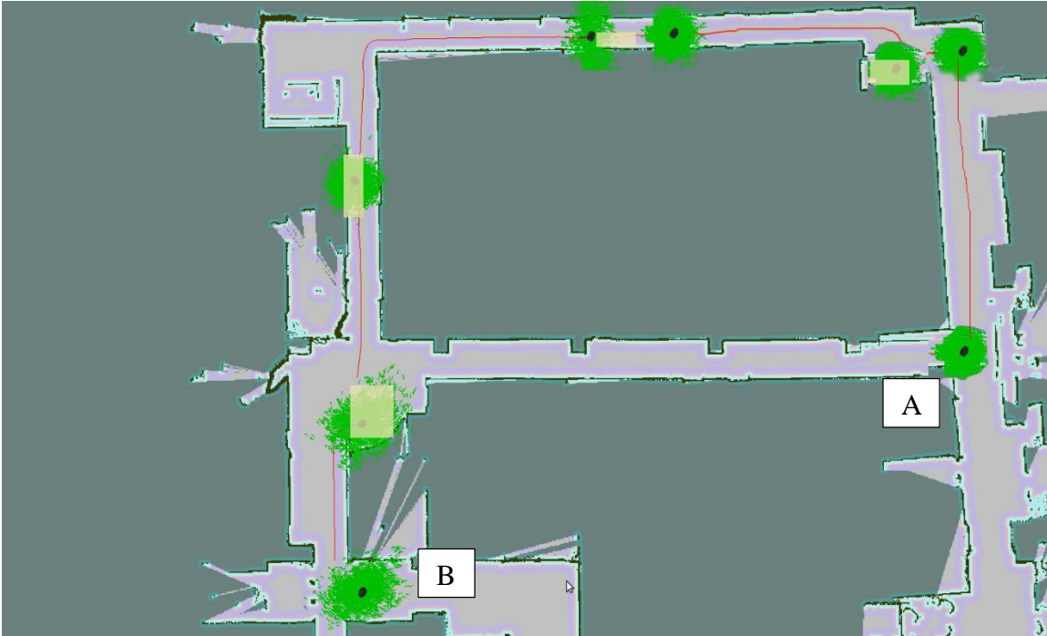
Figure 11. Time lapse of a Create navigating itself through various unknown areas instead of taking the shortest path from A to B. The yellow shaded regions are the areas of interest
