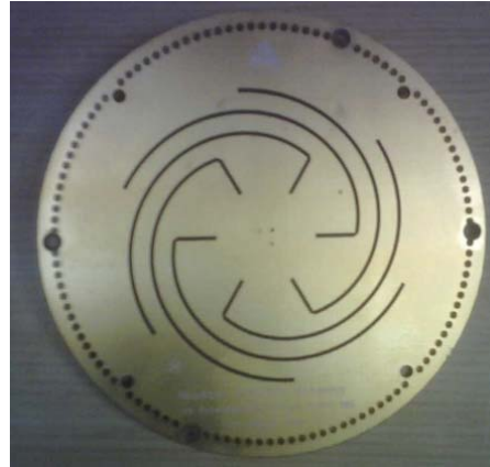
Fig. 3-1: GNSS Fixed Radiation Pattern Antenna Element.
