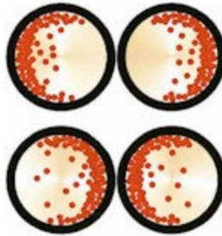
Fig. 1.5 Illustration of Proximity Effect in Closely Conductors
