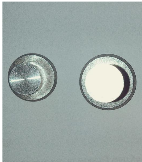
Figure 42. Overlapped the compressed and uncompressed specimens
