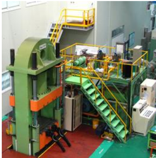
Figure 3. 10,000 tons hydraulic press machine(koteco.co )
