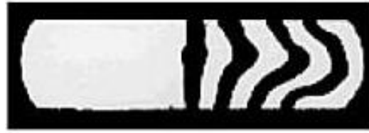
b Lubricated specimen with lather grid pattern
