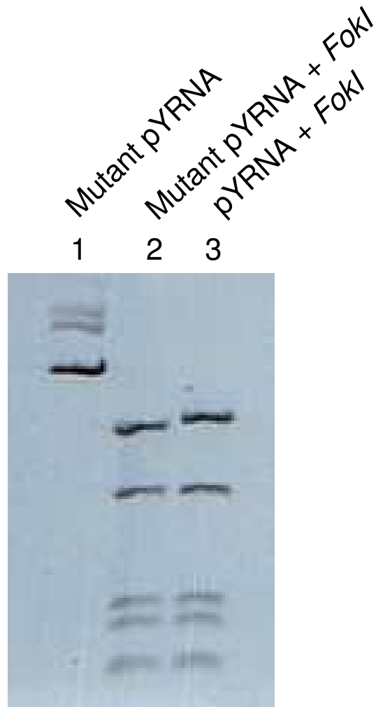
Figure 2.7. Digestion of mpYRNA8 and pYRNA8 plasmids with FokI .
