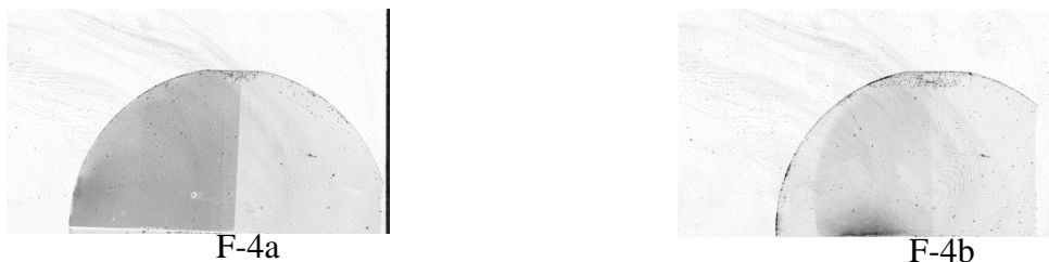
FIGURE F-4: Fluorescence comparison of photo-deprotection efficiency at 260nm and 365nm. The darker region of image F-4a & F-4b corresponds to section of the wafers which was irradiated at 260 nm and 365 nm respectively for different time intervals (1s, 2s, 3s, 14s). The lighter regions correspond to control sections (no irradiation) of the two wafers. The wafers were imaged using Alexa-555 dye.
