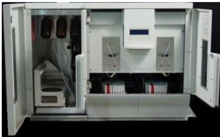
FIGURE G-1: A picture of continuous flow peptide synthesizer manufactured by PerSeptive Biosystems.
