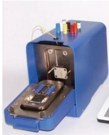
FIGURE 4: Photograph of a potentiosense instrument. The externalized leads of the instrument provide connection between the microelectrodes of the chip and external instruments.
