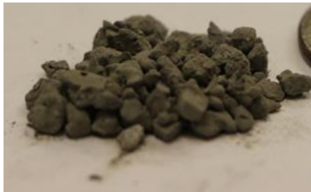
Figure 0-4: Picture of coated LWA
