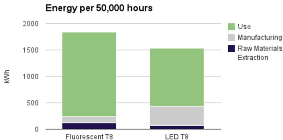
**Figure 2: Total energy consumption for each lighting option, per 50,000 hours of use**
