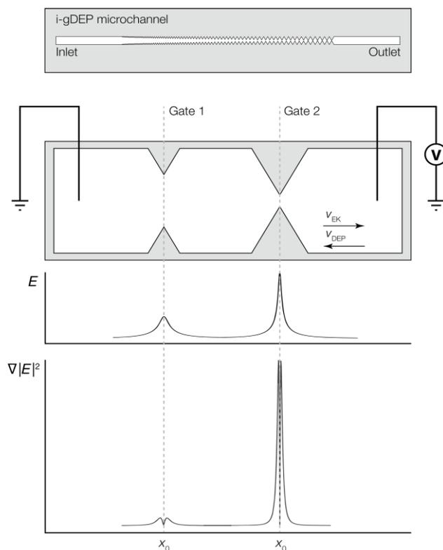
**Figure 1.** A) Diagram depicting concentration of analyte at a gate structure within a g-iDEP microchannel. Peak width is a function of focusing factors associated with electrophoretic velocity ( $v_{EK}$ ) and dielectrophoretic velocity ( $v_{DEP}$ ) balanced with dispersive forces including
