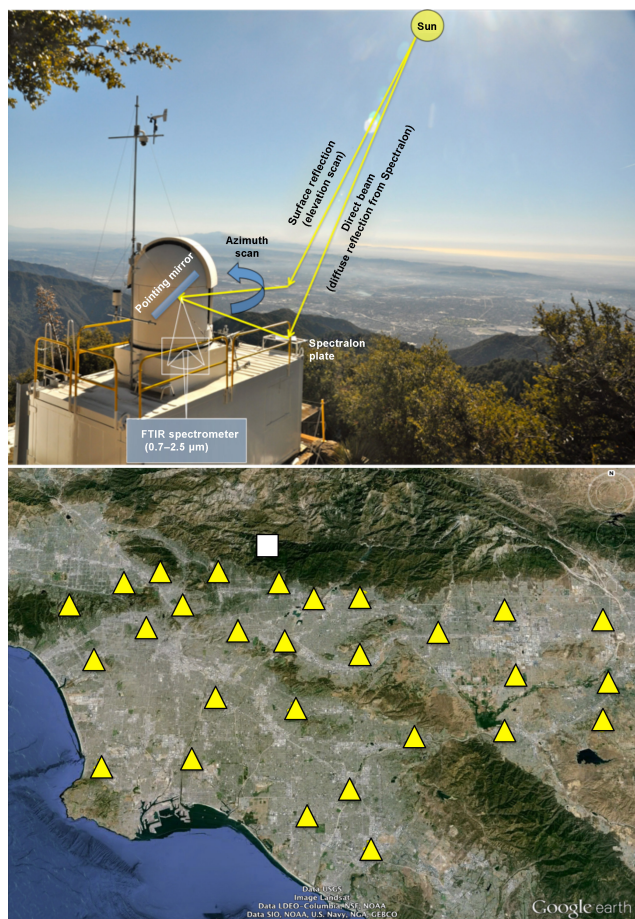
Figure 1. Top: CLARS facility located at 1.67 km above sea level on Mount Wilson, looking over the Los Angeles Basin. Optical paths from direct sun beam and basin surface reflection are shown as yellow lines. Bottom: location of 29 reflection points on Mount Wilson (white square) and in the basin (yellow triangles).
